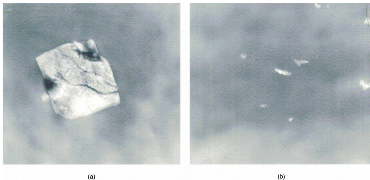
Fig. 4. Ambient temperature unstained TEM images (i.e. negatives) of (a) iPP containing 2 wt% micron-size particles of zinc oxide (i.e. MicroZn), 1\text{ cm} \approx 0.44\ \mu\text{m} which corresponds to a magnification of \approx 23,000\times , and (b) iPP containing 2 wt% nanoparticles of zinc oxide (i.e. NanoZn), 1\text{ cm} \approx 0.29\ \mu\text{m} which corresponds to a magnification of \approx 35,000\times . The surface of the micron-size zinc oxide particles in (a) is smooth and their shape is rectangular. Separate nanoparticles of zinc oxide in (b) have dimensions of approximately 40 nm, whereas the agglomerated particles have lengths of about 150 nm. All samples were extruded at 239\text{ }^\circ\text{C} from a twin-screw micro-mixer.
